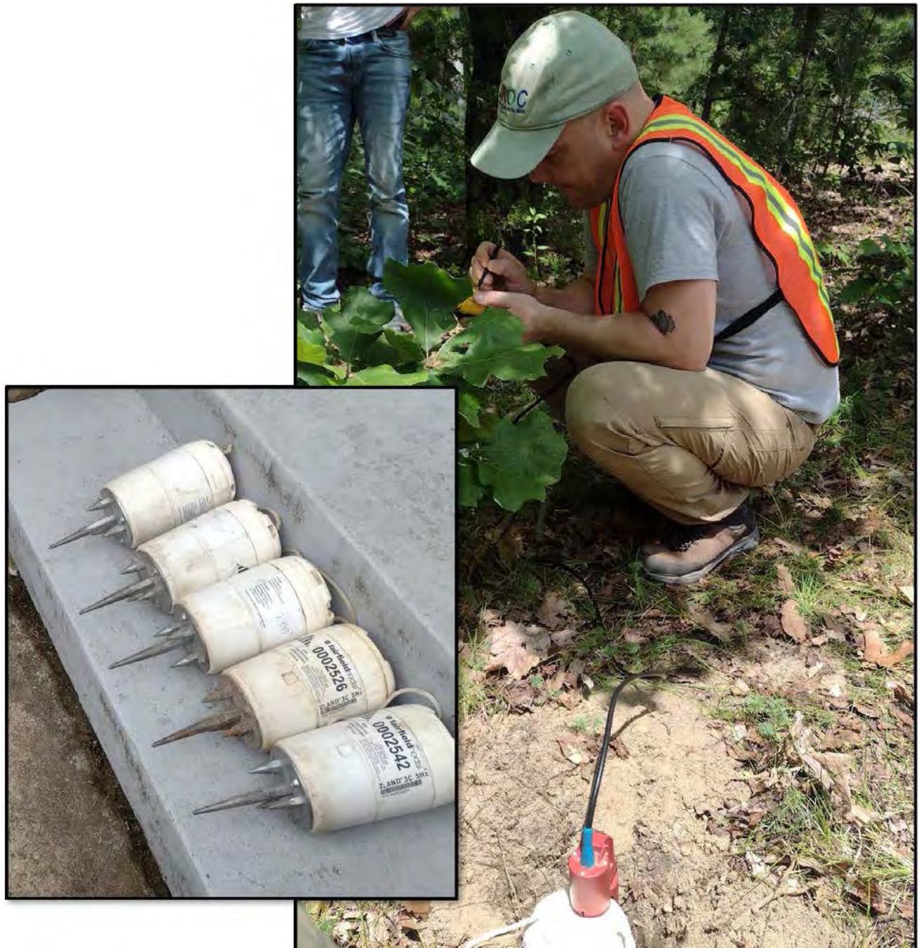
Figure S1: Fairfield ZLand 3C Nodes and deployment. In the larger photo is Hannes Bernhardt (foreground, deployment) and Miguel Endara (background). Ticks were rampant at stations, future studies should ensure participants use proper tick repellent.
